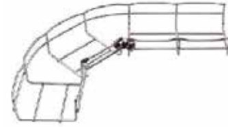
TEL KABLO KANILI 90° YATAY DÖNÜŞ ELEMANI WIRE-MESH CABLE TRAY HORIZONTAL BENDS 90° (H: 35 - 55 - 75 - 100)
